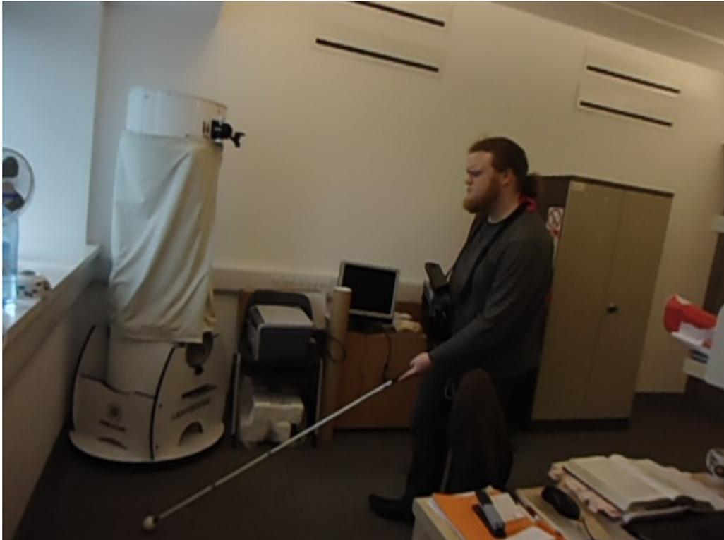
Figure 7.13: Calibrating Kinect-aided navigation system by letting a visually impaired person to walk using it along with white cane
