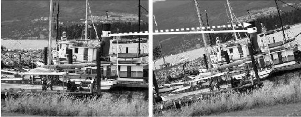
Figure 3.11: Transformation of a point by a homography calculated from feature matches (dotted line) and the ground-truth homography (solid line). This is a failure for  $\tau = 2$  pixels.
