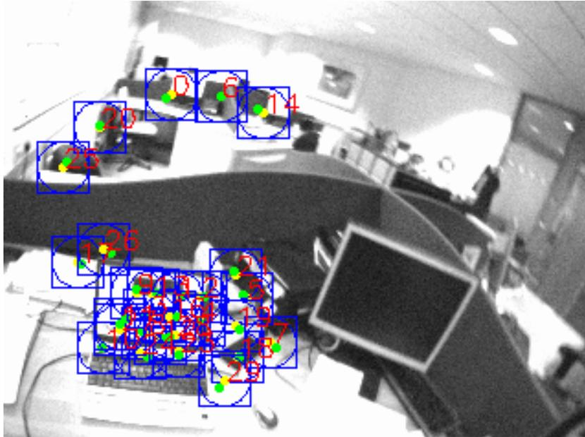
Figure 4.12: Incorrect data association. Notice where the initial position of Feature #14 (as well as other features) in Figure 4.10(b) was and where it is being predicted and matched in later frames.
