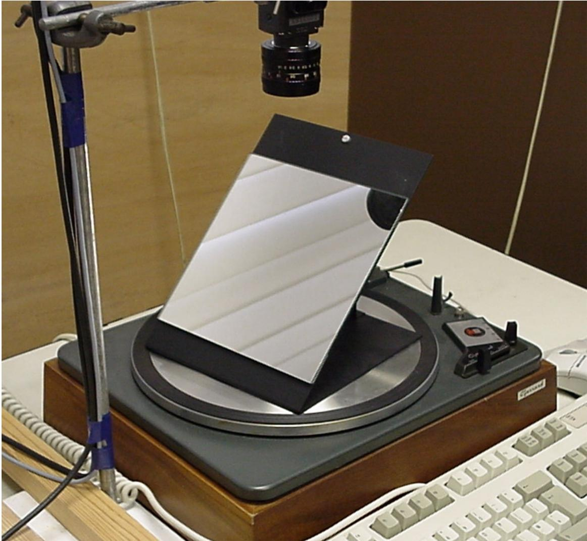
Figure 3.9: Photograph of the experimental apparatus used to implement a periscopic stereo imaging system.
