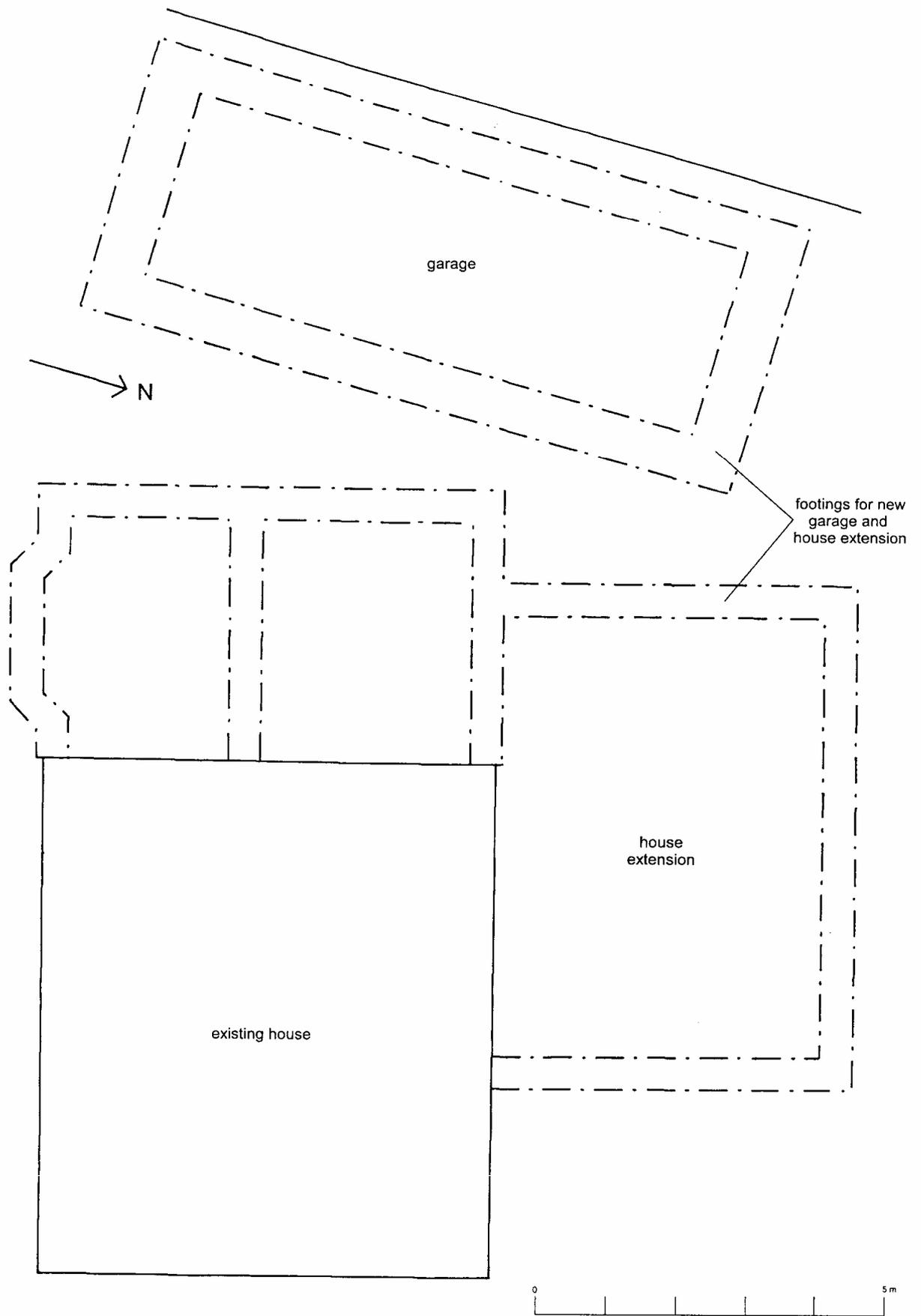
Fig 1 Plan of footing trenches for house extension and new garage
