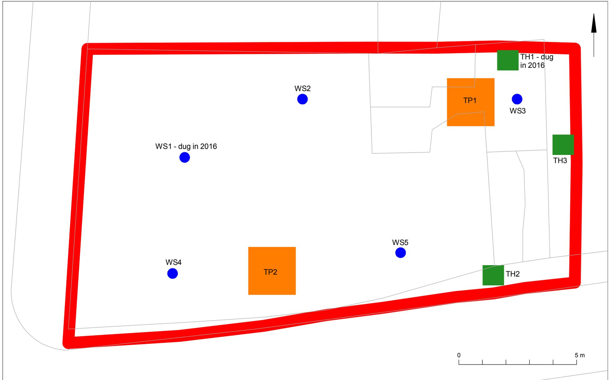
Fig 2 Proposed location of evaluation test-pits (TP1-TP2) and location of window samples (WS1-WS5) and trial-holes (TH1-TH3) to be monitored
