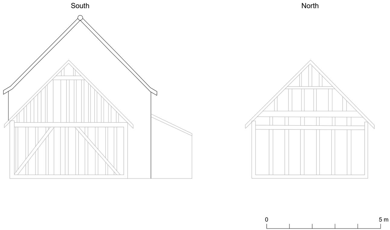
Fig 7 Frame drawings of the fore-building prior to its demolition (taken from pre-existing architects drawings).
