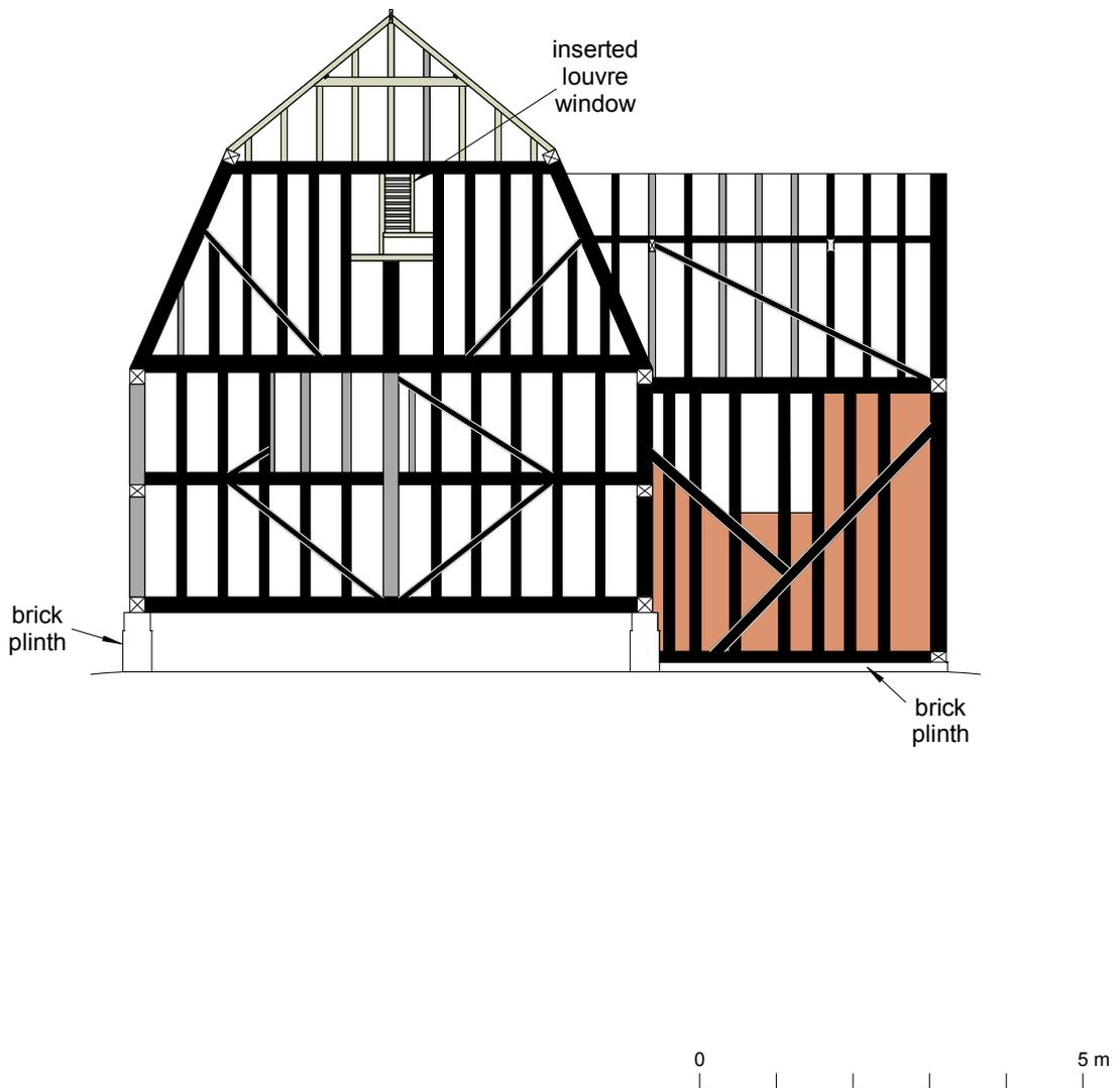
Fig 9 Frame drawing of the north-west wall to the Grain Barn, indicating the locations of original, re-used and replacement timbers.
