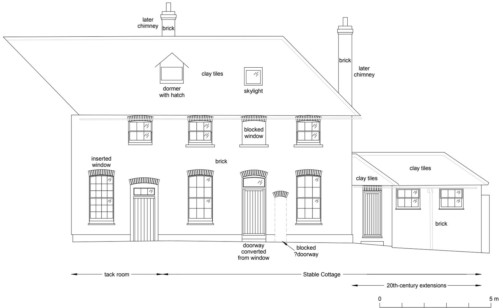
Fig 9 Structure 1/2, 18th-century stable block south-west elevation.
