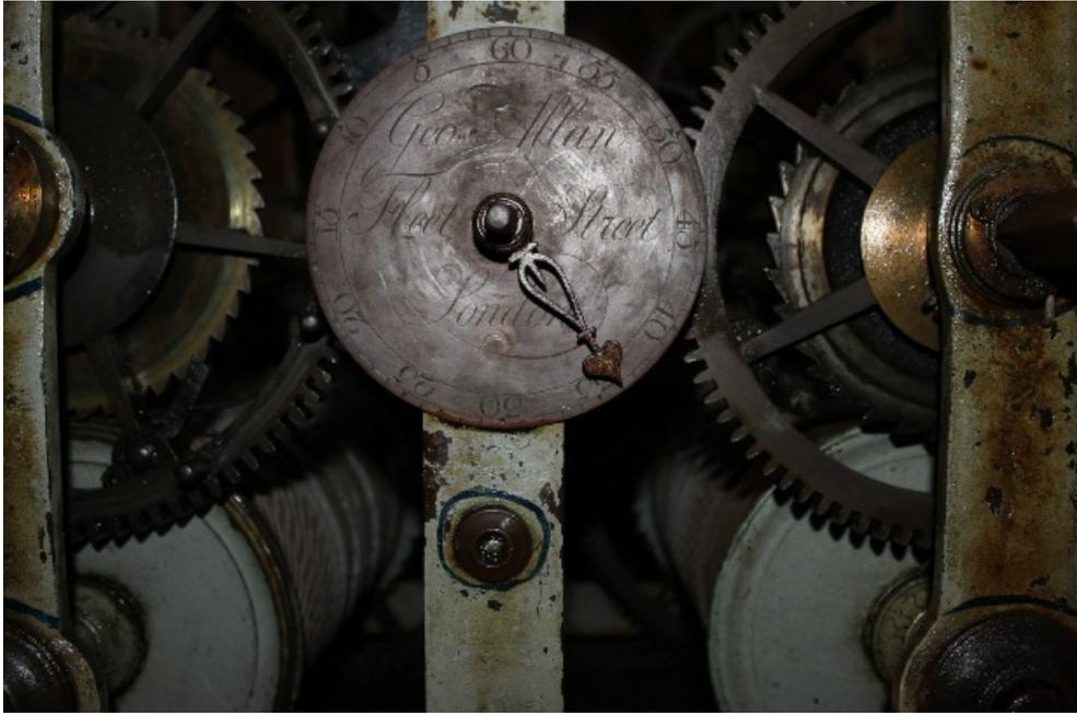
**Plate 31** Structure 1/2, detail of the clock mechanism below the cupola bearing the manufacturer's details: Geo[rg]e Allan, Fleet Street, London
