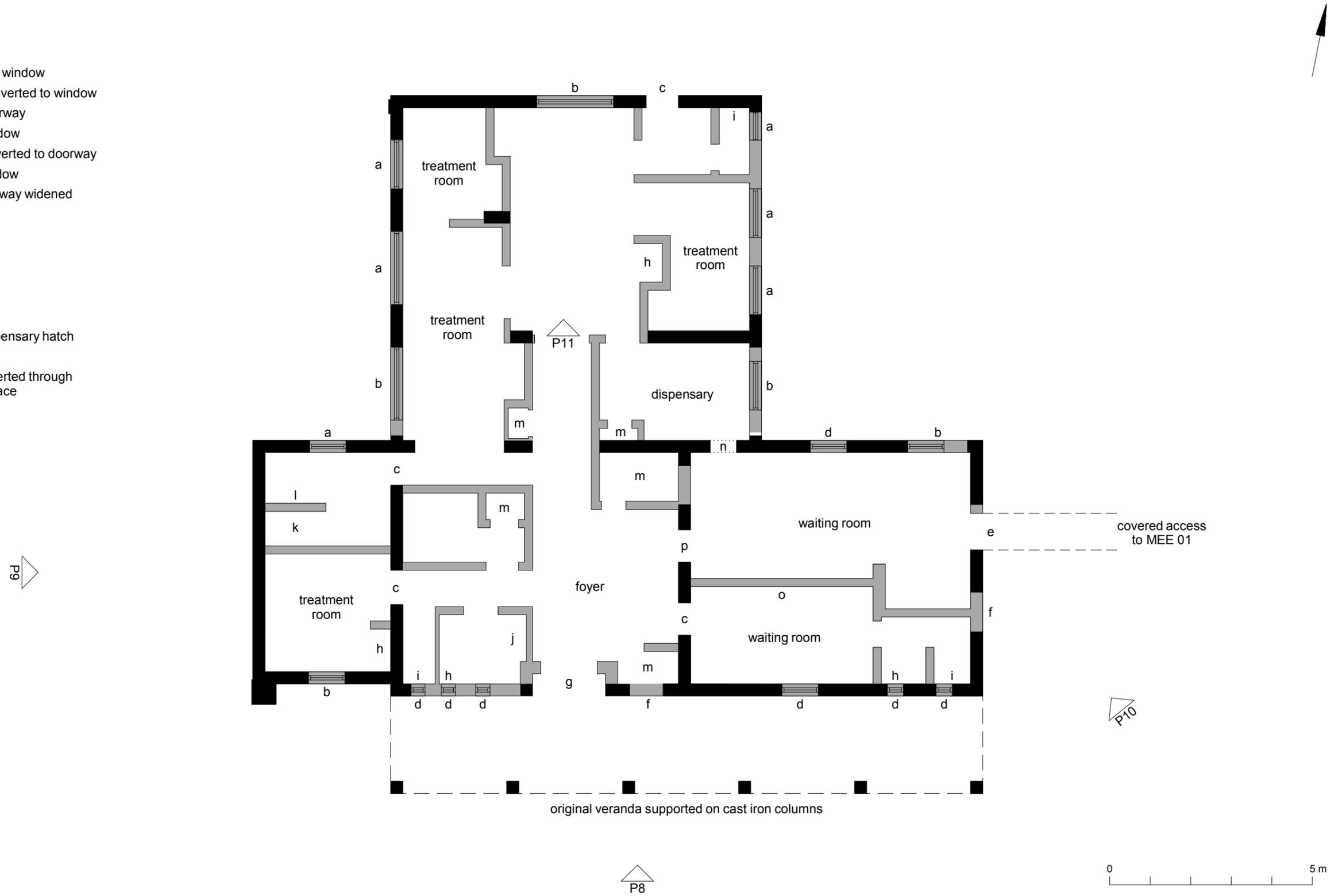
Fig 29 MEE 03: floor plan of the former Meeanee Barracks Guard House, with original fabric shown black and medical centre alterations shaded grey. The location and orientation of photographs included in this report are indicated by the numbered arrows.
