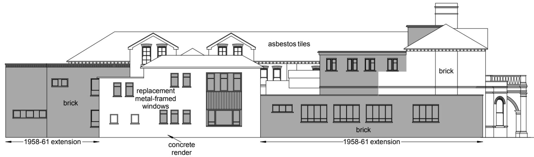
Fig 40 MEE 17: north elevation of the Meeanee Barracks Officers' Mess and Quarters, with alterations shaded grey.
