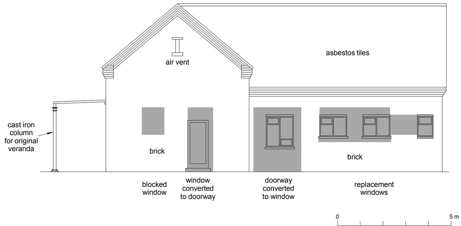
Fig 32 MEE 03: east elevation of the former Meeanee Barracks Guard House, with alterations shaded grey.
