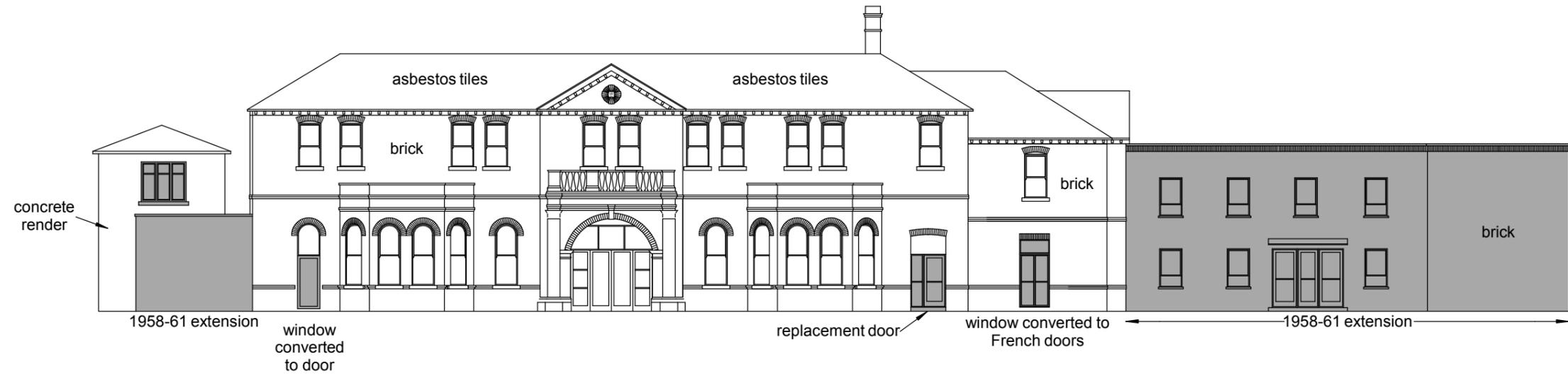
Fig 37 MEE 17: west elevation of the Meeanee Barracks Officers' Mess and Quarters, with alterations shaded grey.
