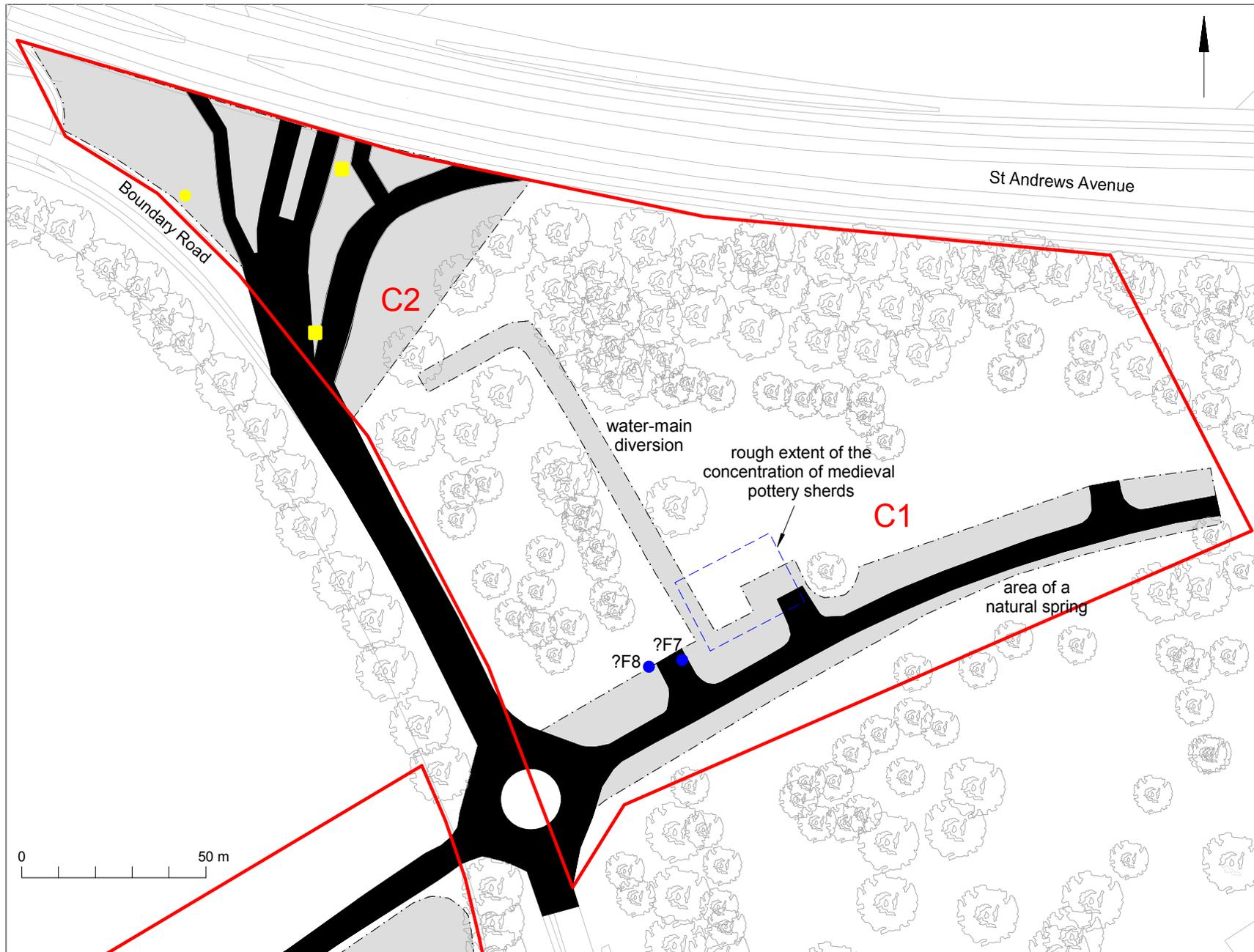
Fig 9 Area C: the areas shaded grey are where the topsoil stripping was observed.
