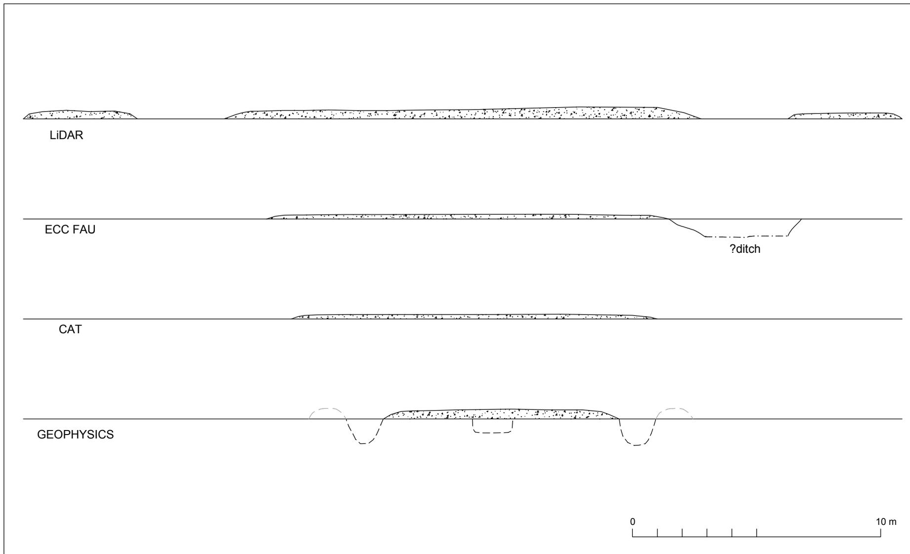
Fig 6 Idealised sections showing the construction of Barrow A based on different strands of evidence.
