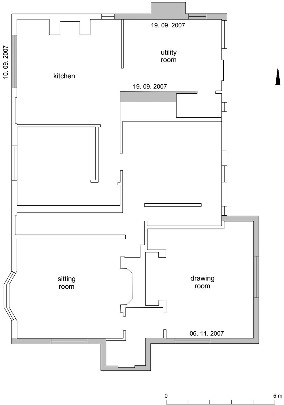
Fig 2 Plan of farmhouse foundations, showing observed footings.
