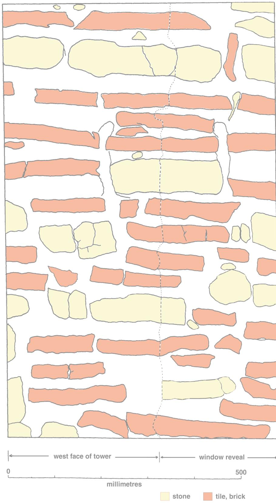
Fig 2 The window reveal and adjacent west face.
